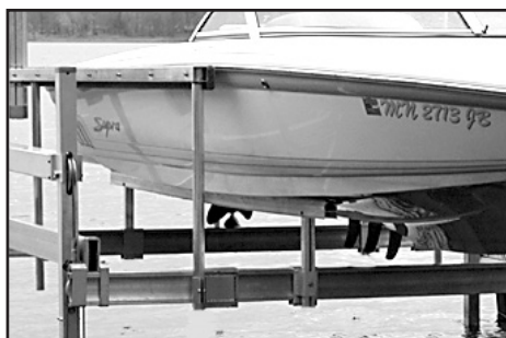
Fig. 37b - Bunk height recommended for inboards - The bunks are spread wide and the hull is lifted so that the running gear on an inboard can pass over the main lift beam without making contact.
