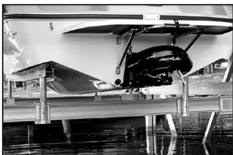
Fig. 37a - Ideal bunk placement - Note that the bunks are spread out to the widest position on the boat hull. They sit nicely into the contour of the hull and the keel has plenty of clearance above the main lift beam. If possible, this is the most ideal bunk placement for non-inboards.
