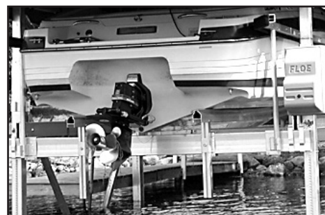
Fig. 37c - Less desirable bunk placement - Ideally in the above example, the lift bunks would have been positioned wider as in Figs. 37a & b . Doing so would have allowed the bunks to be set higher, preventing the vertical tubes from sticking so far below the main lift beam.
