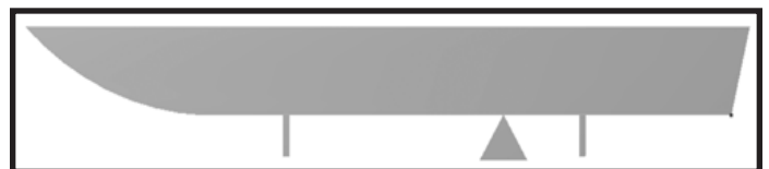
Illustration C: shows a boat's center of gravity (CG) improperly positioned so that it extremely overloads one of the main lifting beams.
