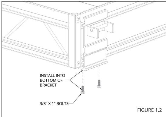
TORQUE BOLTS TO 6 FT-LB MAXIMUM (FIGURE 1.3). AFTER REMOVING EACH BOLT THAT IS INSTALLED IN THE RAMP HOOKS, INSTALL THE RAMP ONTO THE BRACKETS (FIGURE 1.4).
